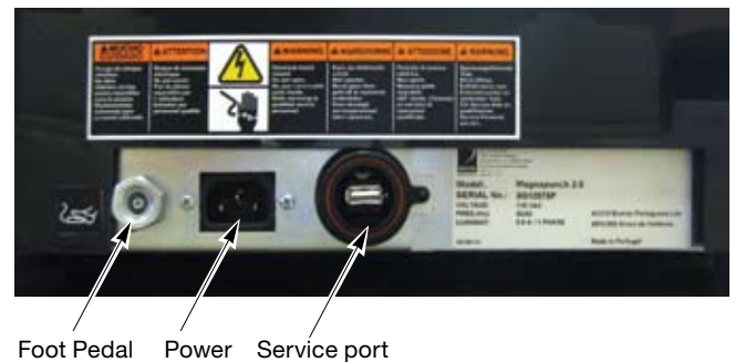
Figure 5. Connections on Back of Magnapunch 2.0.
