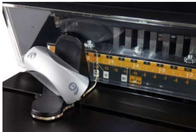
Figure 9. Edge Guide Unlocked.
