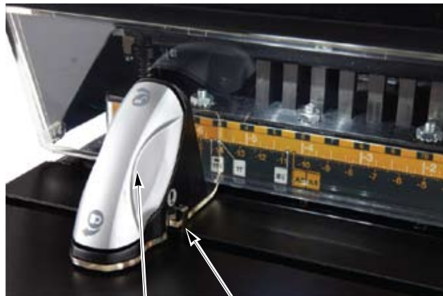
Edge Guide adjustment handle Tabletop Trigger
